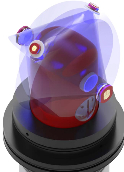
Four UV LEDs illuminating the CT cell
