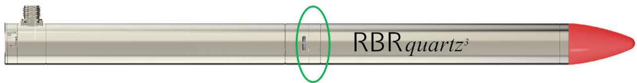
Location of the coupling piece on the RBRquartz 3 APT
