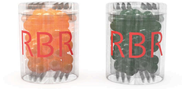
Fresh (orange) and saturated (green) desiccant capsules
