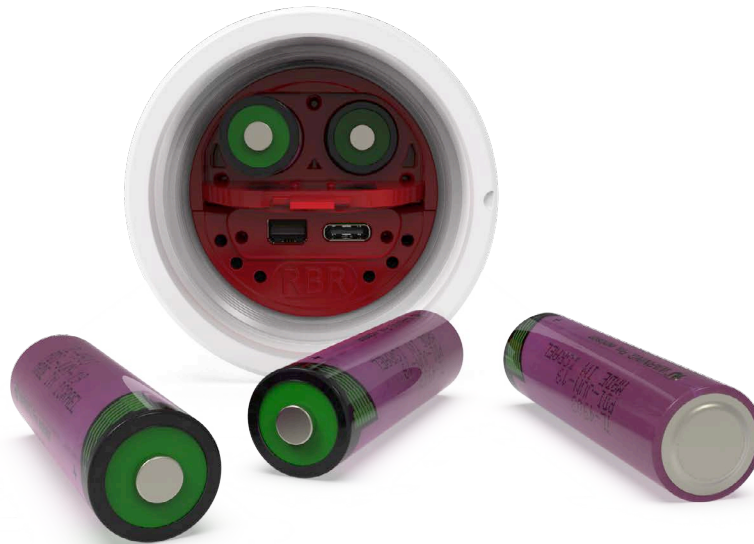
RBR standard instrument with batteries removed
