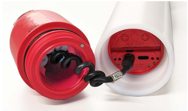
Open instrument with a connectorised end-cap
