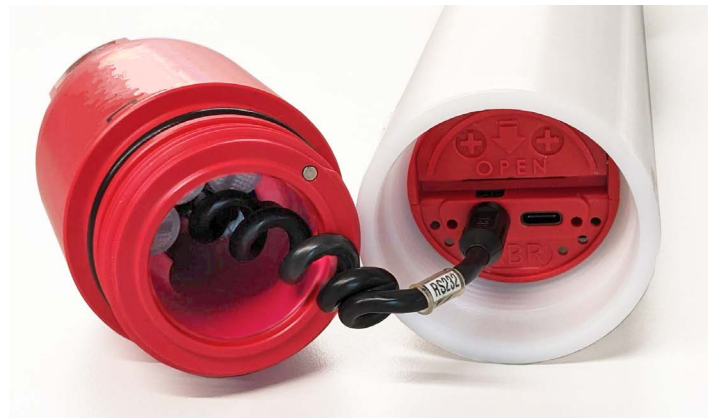
Open instrument with a connectorised end-cap
