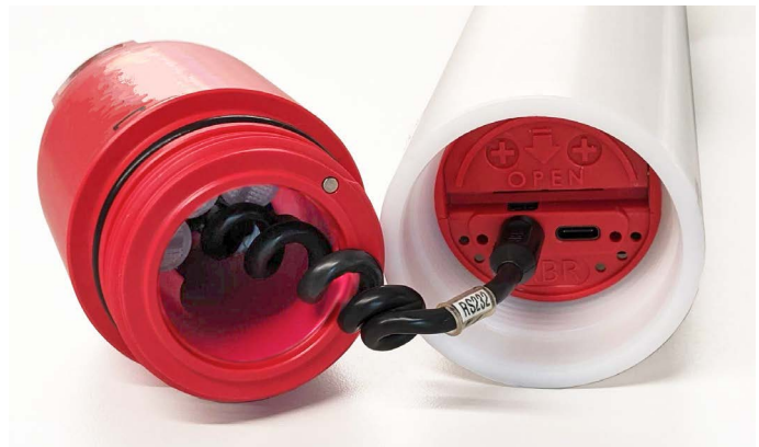
Open instrument with a connectorised end-cap
