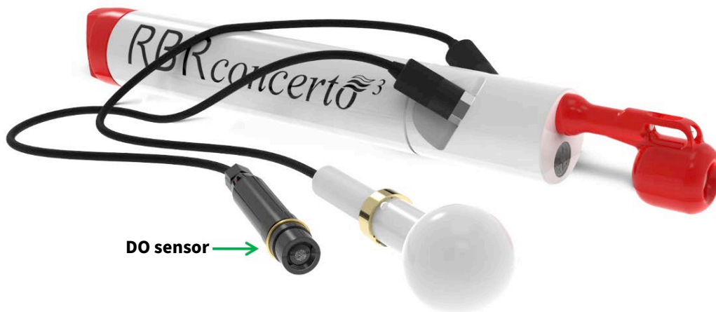
RBRconcerto 3 C.T.D.DO.PAR with a DO sensor (OxyGuard)
