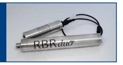
The RBRduo BPR uses proven proprietary technology and a Digiquartz® transducer to achieve 10ppb depth resolution with sub-second integration times. The short integration times consume less power during sampling resulting in significantly longer deployments between battery replacements. User selectable integration time for each reading means you can adjust the resolution to your measurement needs.
