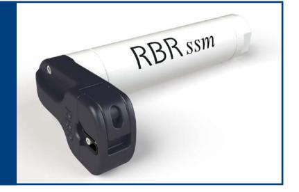
The MLM-1000 consists of two major components; the head end modem (HEM) and the subsurface modem (SSM). Each instrument on the mooring line system is connected to an SSM, which communicate inductively with the HEM (and host) through the mooring cable.
