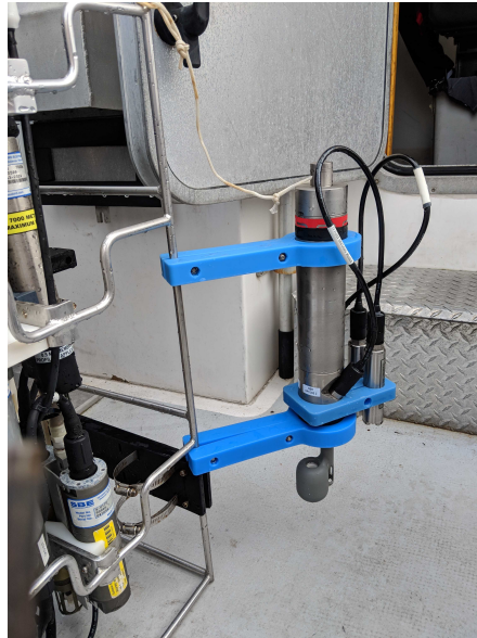
Fig. 2 RBRconcerto and two RBRcoda T.ODOs mounted on SBE cage with clamps for vertical profiling.
