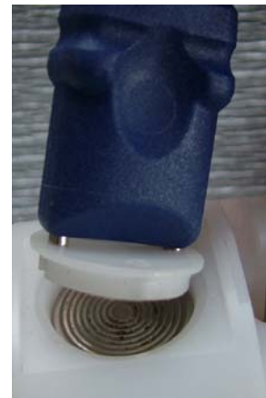
Figure 4. Flipping off the cover from a pressure transducer
