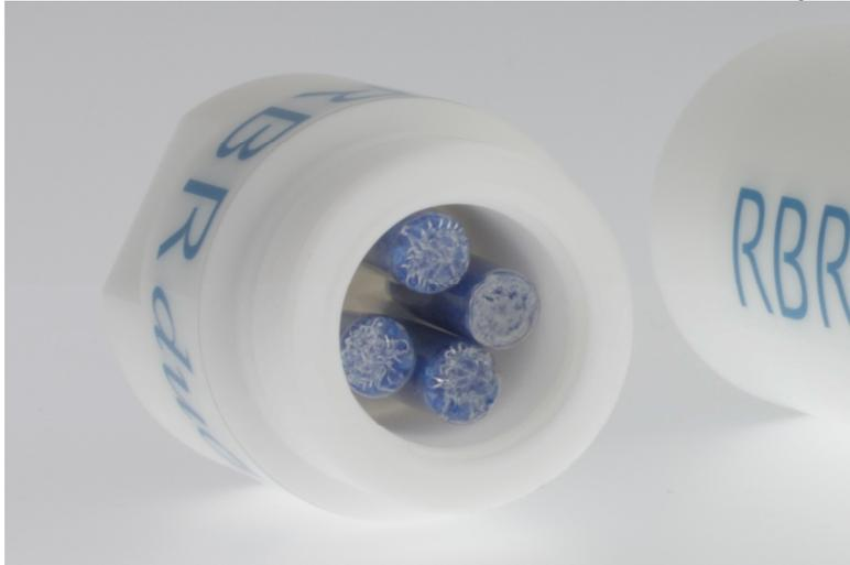
Placement of the capsule packs for the RBR*virtuoso*, RBR*duo* and RBR*concerto* is the same. Simply remove the bottom end cap (i.e.: the non-sensor end) and place (2) to (4) packs into the desiccant holder.
