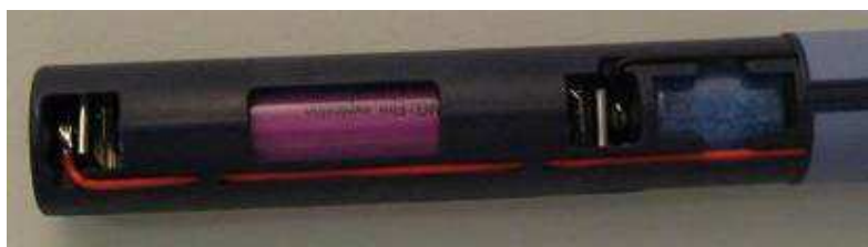
Fig. 3 Keyhole opening for battery removal
