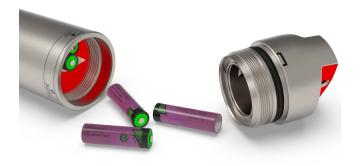
Open instrument with a standard end-cap
