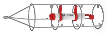
3. To pause logging, turn the battery end-cap to the **PAUSE** position. The instrument will vibrate with **three short pulses** to indicate it has stopped sampling.
