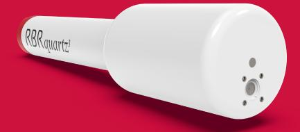
The RBRquartz³ Q uses an integrated Paroscientific Digiquartz® pressure sensor. It offers a flexible measurement schedule, standard and burst sampling, large memory, and sufficient power for extended deployments. The RBRquartz³ Q offers a variety of interfaces, including an internal USB-C port and an optional external port, which can be configured as USB, RS-232, or RS-485.
