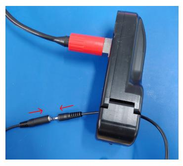
MLM test loop through ferrite holder
