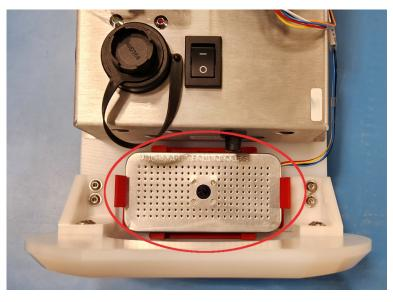
**Desiccant canister fully inserted**
