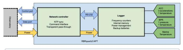
You do not need to open your instrument to connect it to your network. Connect your terminal to the MINK port located outside the instrument body using a compatible MINK cable. The instrument will appear on your network.
