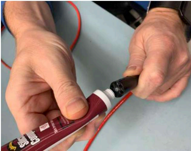
Lubricating a connector
