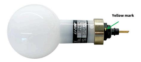
Always align this yellow mark with the tab on the side of the cable connector when connecting the sensor to its cable.
