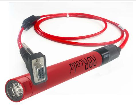
RBRcoda<sup>3</sup> D with an RS-232 cable, DB9-F connector
