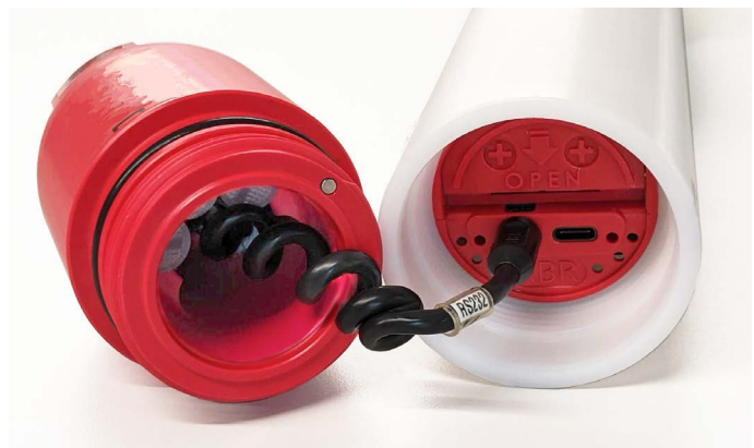
Open instrument with a connectorised end-cap
