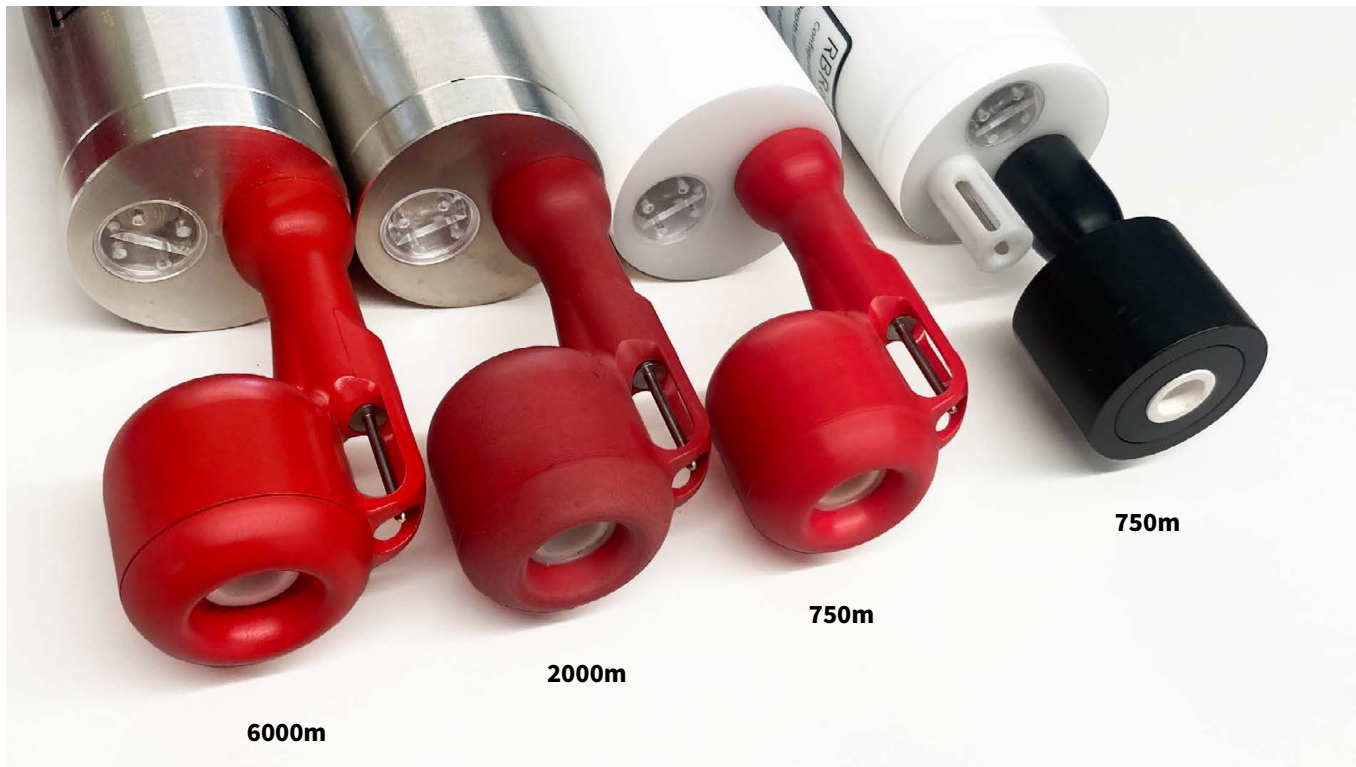
750m-, 2000m-, and 6000m-rated conductivity cells
