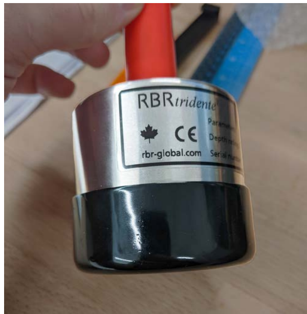
RBRtridente with its storage cap on
