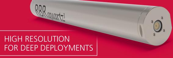
The RBR*quartz<sup>3</sup>* BPR (Bottom Pressure Recorder) uses an integrated Paroscientific Digiquartz<sup>®</sup> pressure sensor for the bestin-class initial accuracy, resolution, and low drift performance. The RBR*quartz<sup>3</sup>* BPR is intended for tsunami detection, tide monitoring, long-term water level studies, and high-resolution depth sensing in ROVs and AUVs.
