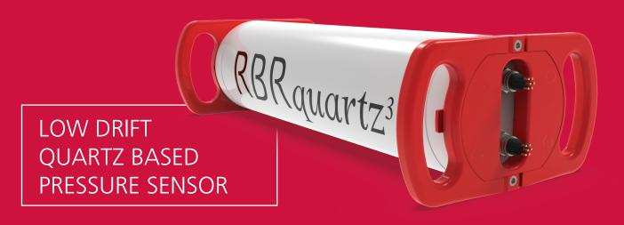
The RBRquartz<sup>3</sup> Q|plus tide and wave logger integrates the Paroscientific Digiquartz<sup>®</sup> pressure sensor for best-in-class initial accuracy and low drift performance. Intended for long-term autonomous or realtime observations of water level, tides and waves, this incredibly stable pressure sensor in the RBRquartz<sup>3</sup> Q|plus can resolve small changes over long deployments.
