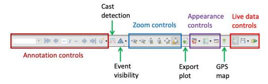
Click the **Side data panel** button to toggle on and off the data panel to the right of the plot. It shows the file location that will be used to capture samples, the number of samples collected, the values of the last received sample, and the currently selected sample.
