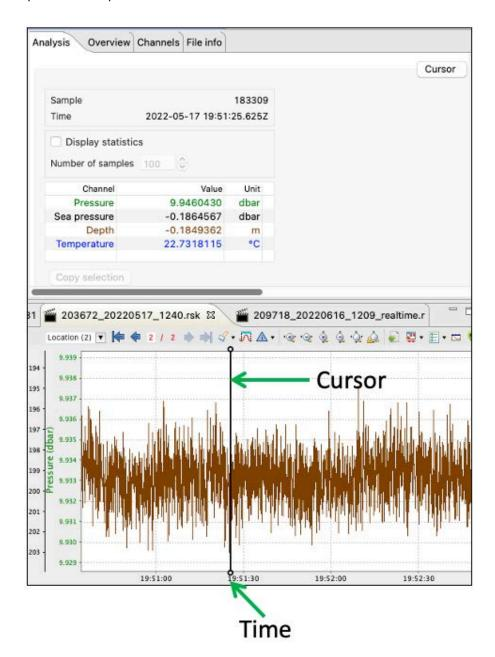
Select **Display statistics** checkbox to determine the average value and standard deviation over a range of samples. Change the number of samples to average using the up and down arrows.
