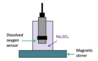
4. Record the data for at least 30 minutes. This is the 0% oxygen concentration calibration point.
