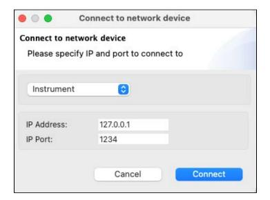
(i) For the microsalinometer, the port number must be 23.
