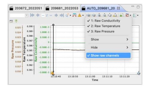
By default, the data are plotted by time. Use the **Toggle depth plot** button to switch to the plot-by-depth mode.
