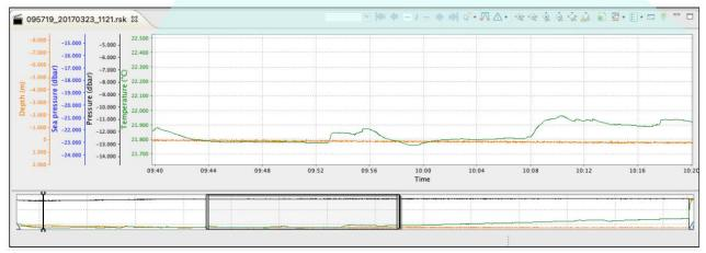
5. To keep all your data within the viewing window, click the **Toggle auto-ranging** button . When it is on, all profiles within the selected time section maintain their optimal vertical zoom.
