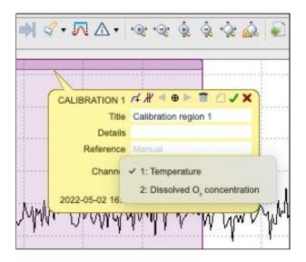
e. Press **Enter** on your keyboard or click **Save** on the tooltip to save the calibration region. A section for this calibration region will open under **Cursor**.
