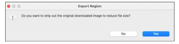
6. Select **No** to maintain the full binary values and retain the option of recalibration in the future. The clipped dataset will open in a new tab in the **Plot** window.
