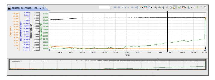
There are three ways to apply changes to the horizontal scale. The first two will auto-range your chart, ensuring the entire vertical domain is visible. The third approach will retain the latest vertical scaling of the original interval.
