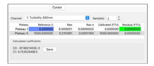
b. Click **Save** to write the coefficients to the instrument. The instrument must be connected to Ruskin.
