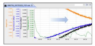
3. To pan one of the channels vertically, click a value on the vertical axis for that parameter (in the example below, sea pressure) and move your mouse up and down.
