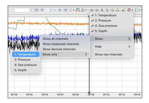
Select **Show raw channels** to display measured data with no calibration equations applied.
