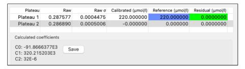
b. Click **Save** to write the coefficients to the instrument. The instrument must be connected to Ruskin.
