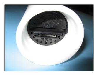
Closing the logger is exactly the reverse of opening it. Remember to keep the O-rings clean and avoid scratching the O-ring mating surfaces. Carefully inspect the O-rings, as described in the Inspecting the O-rings section (p.10), before deploying the logger. Do not use excessive force when tightening the end cap; hand-tight is quite sufficient, as the seal depends upon the O-rings, not the end cap tightness.
