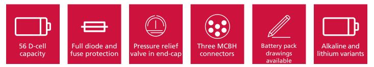
The RBR*fermata* prolongs the life of all deployments by providing 1kWh of power to any underwater instrument.For standard RBR instruments, this is approximately a 40x improvement to our standard battery carriage capacity. Drawings for the battery packs are available to aid local sourcing, particularly in the case of lithium packs (which further increase the capacity to 1.5kWh).
