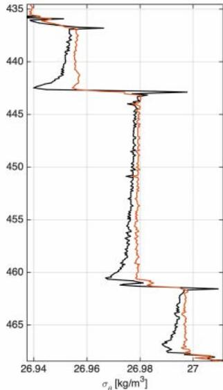
Example of artificial density inversions due to thermal mass errors (black) in a profiling float.
