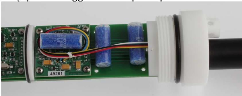
Placement of the capsule packs in the XR and XR(X) loggers depends on the number of sensors used as this will reduce space. The above image shows possible places
