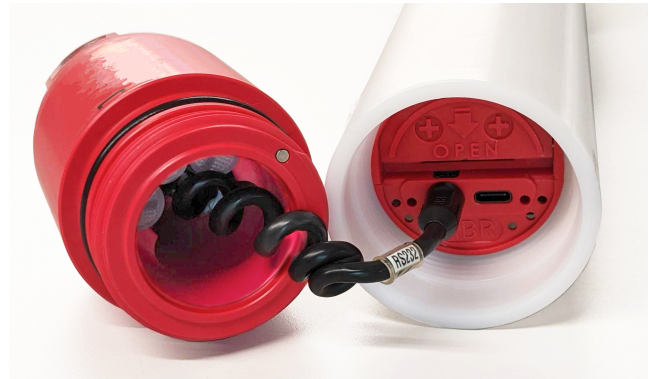
Open instrument with a connectorised end-cap
