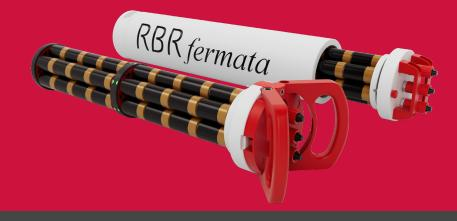
The RBRfermata battery canister extends deployments of all instruments by providing up to 2.8kWh of energy to any underwater instrument, which is about forty times greater than our standard battery carriage capacity. Housing 48 individual D-cells and hosting three MCBH connectors. An innovative battery carrousel coupled with quick-release or low-profile handles facilitates simple, tool-free battery replacement.
