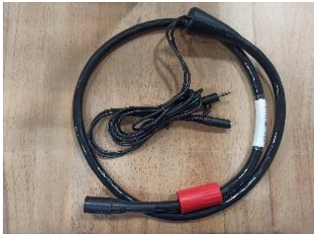
Fig. 5. MLM test loop cable
