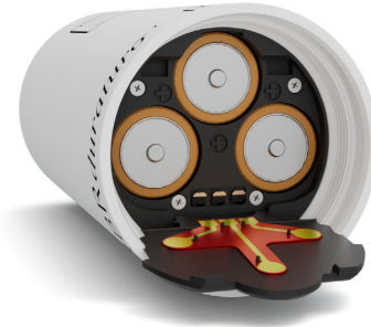
Fig. 8. Location of the battery carriage
