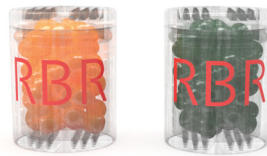
Fig. 11. Fresh (orange) and saturated (green) desiccant capsules
