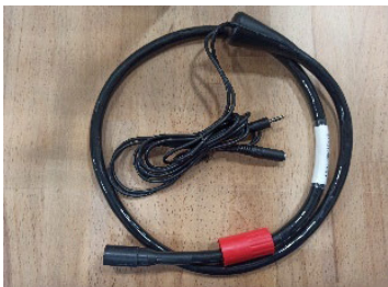
Fig. 8 . MLM test loop cable
