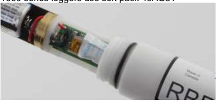
Fold the soft pack on one (length) edge to make it easier to place the desiccant inside the logger. Note the fold in the soft pack in the above image.
