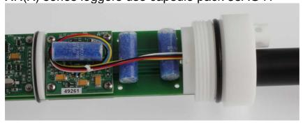
Placement of the capsule packs in the XR and XRX loggers depends on the number of sensors used as this will reduce space. The above image shows possible places
