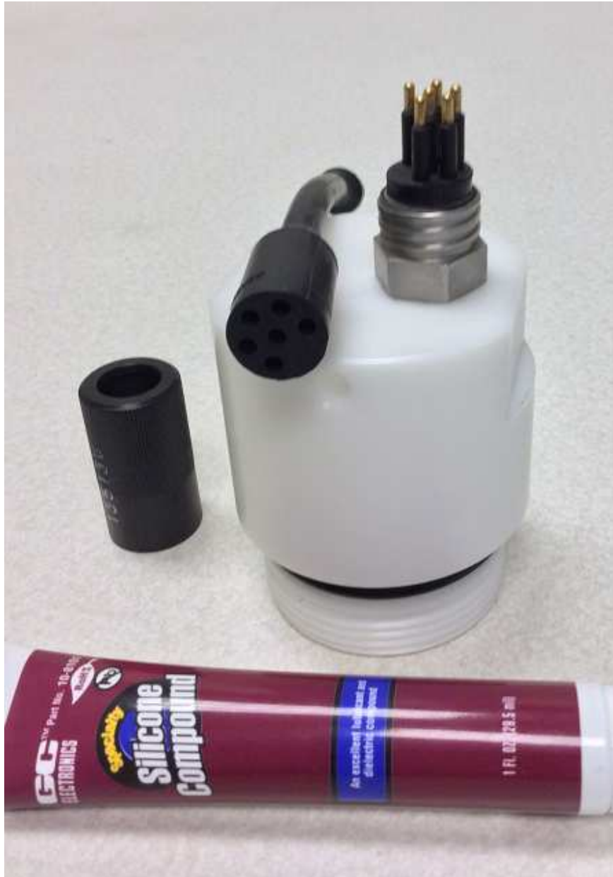
RBR supplied o-ring and connector grease
